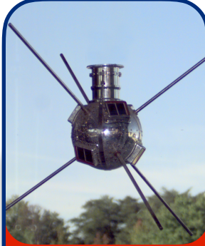
VANGUARD 1— U.S.A. 1ST SATELLITE TO RUN ON SOLAR POWER
